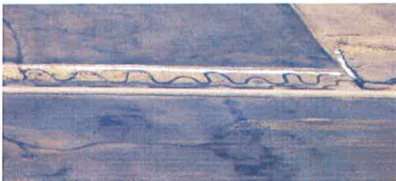
Meandering Channel w/ set back levy – County Road #61, Springbrook Twp, Kittson County
